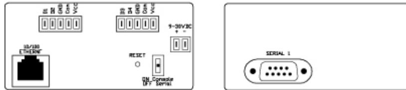
IOLAN SDS1 TD2R2 – 2 Digital I/O, 2 Relay outputs and 1 RS-232/422/485 Serial Port
